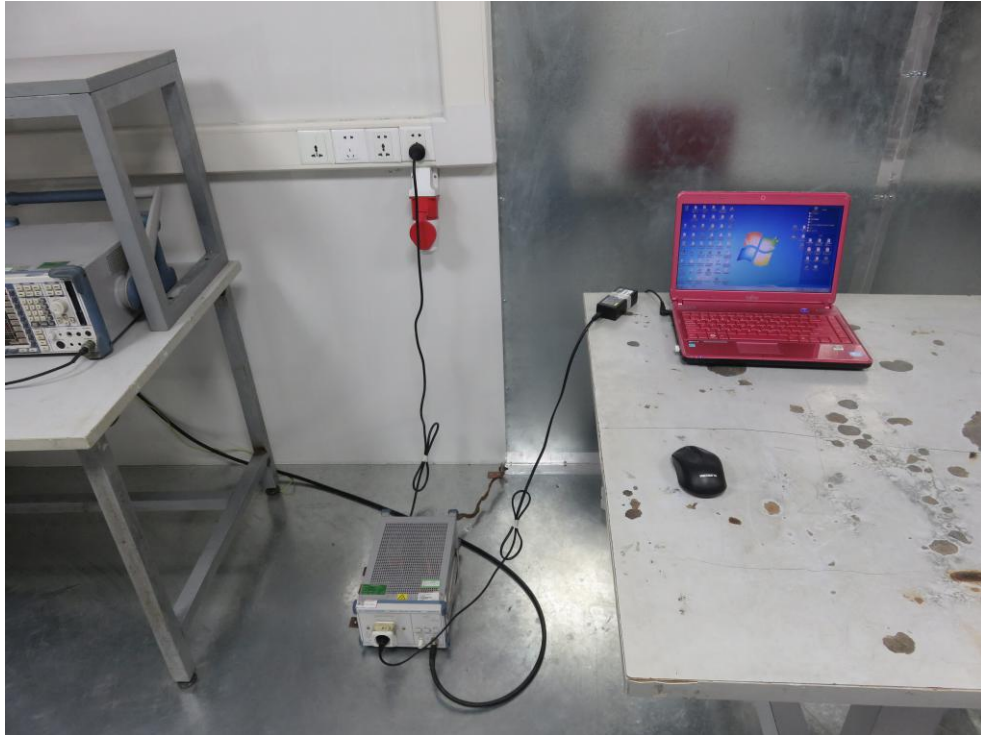
Photo of Conducted Emission Measurement
