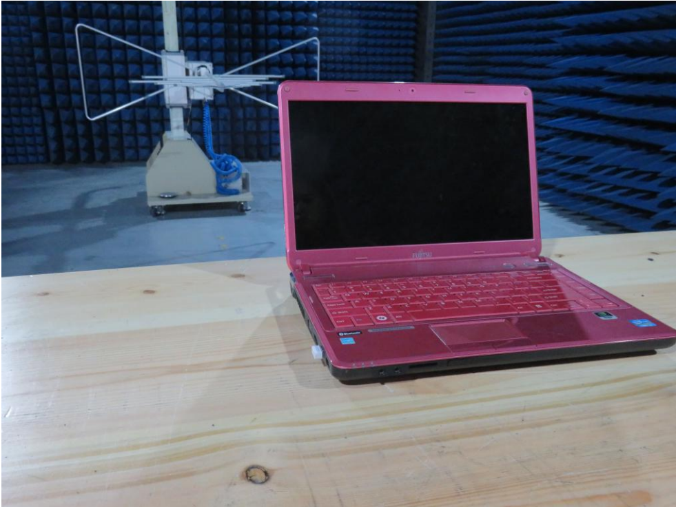
Photo of Radiation Emission Test
