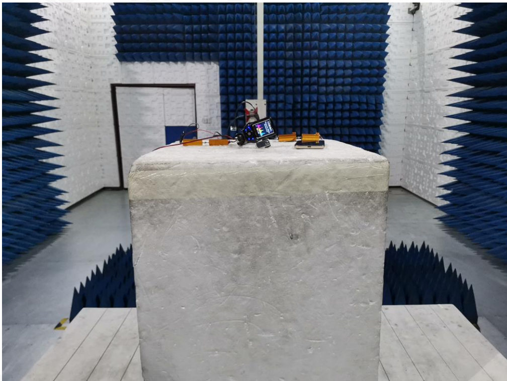
RADIATED EMISSION TEST SETUP ABOVE 1GHZ
