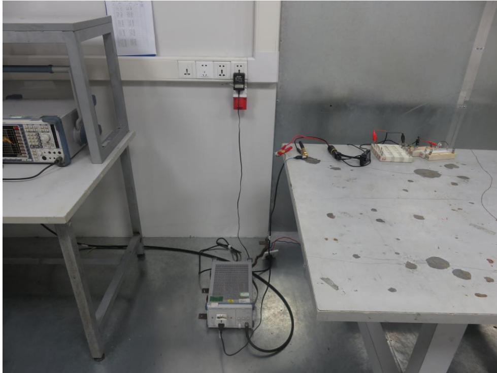
Photo of Conducted Emission Measurement
