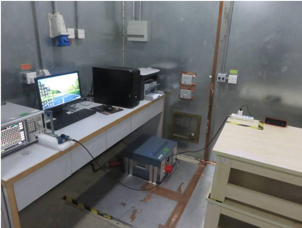
FCC RADIATED EMISSION TEST SETUP
