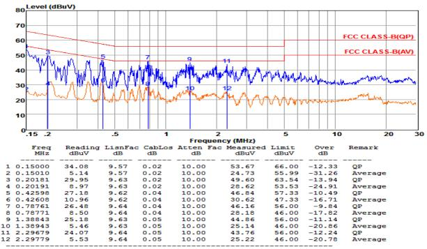
Remarks: 1. Measured = Reading + Lisn Factor +Cable Loss+Atten\_Fac.
