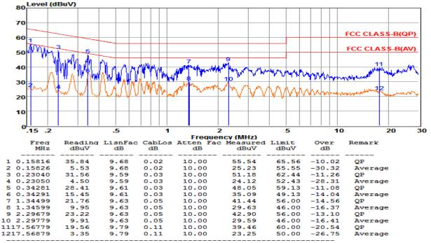
Remarks: 1. Measured = Reading + Lisn Factor +Cable Loss+Atten\_Fac. The emission levels that are 20dB below the official limit are not reported.
