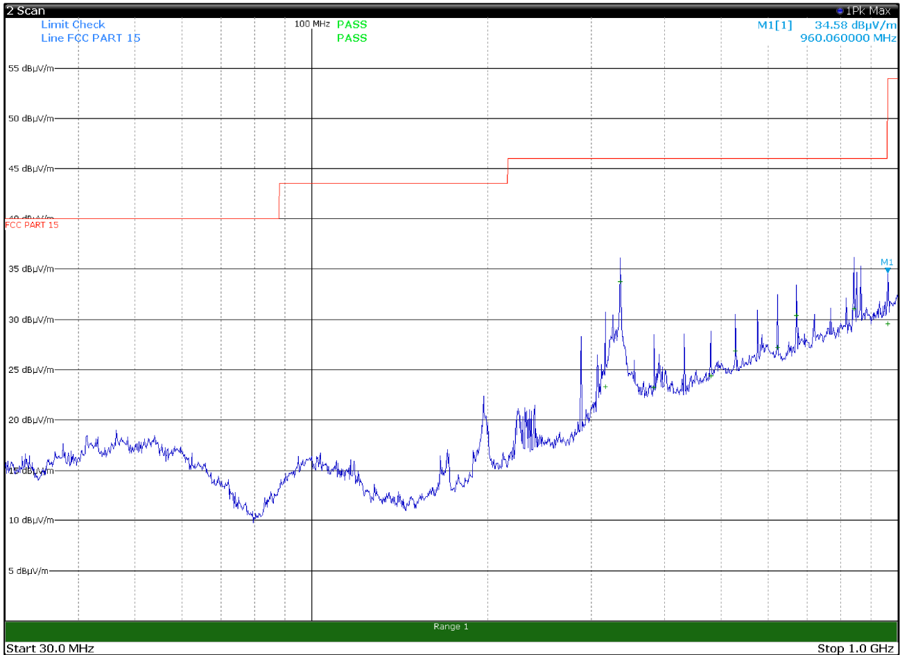
Figure 8.3-8: Radiated spurious emissions for antenna in vertical polarization, mid channel
