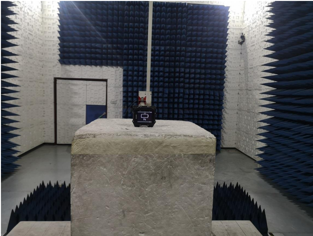
RADIATED EMISSION TEST SETUP ABOVE 1GHZ
