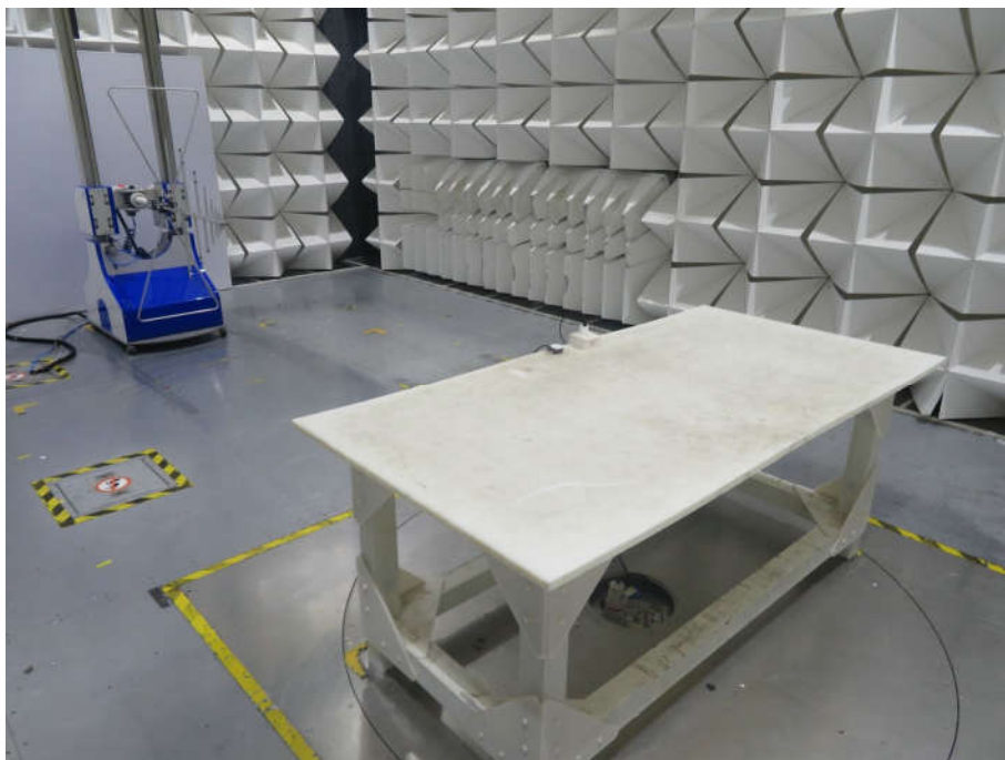
Radiated spurious emission Test Setup-2 (30MHz~1GHz)
