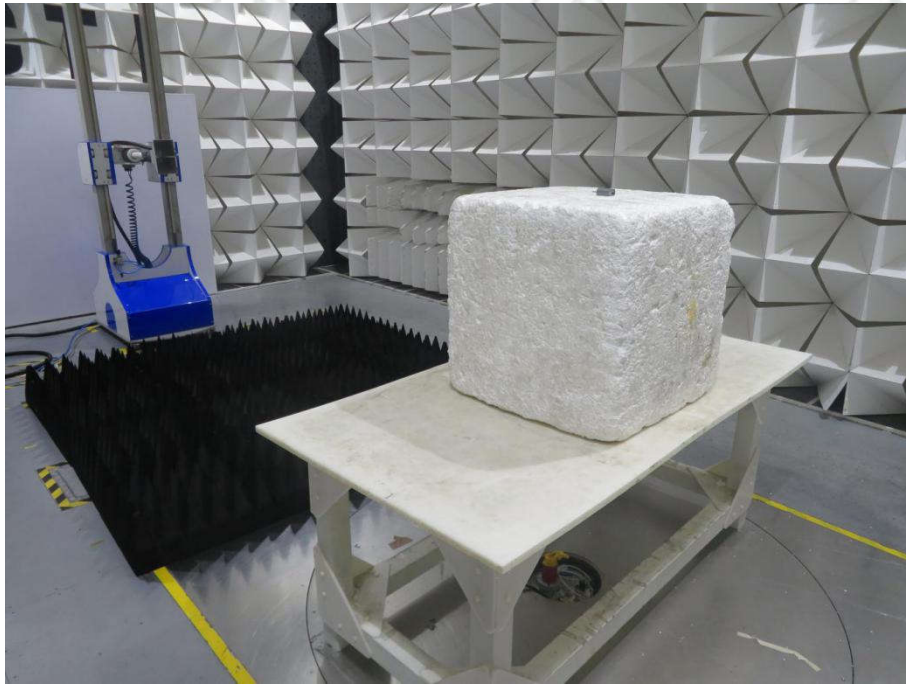
Radiated spurious emission Test Setup-3(Above 1GHz)
