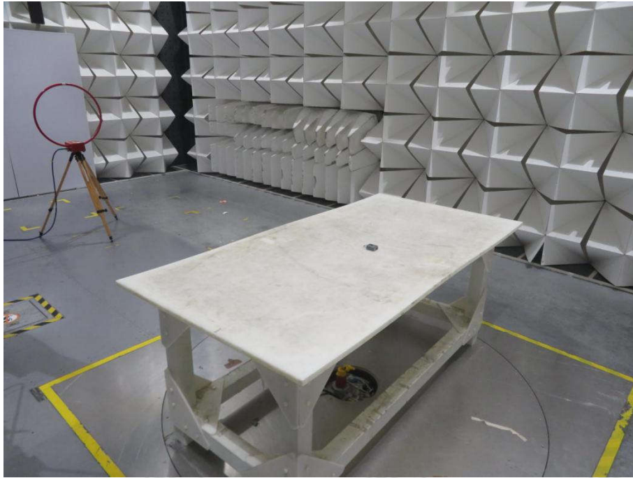
Radiated spurious emission Test Setup-1(9KHz-30MHz )
