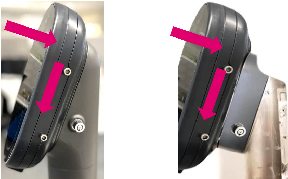
Figure 37: Rugged Validator Mounting on Cradle
