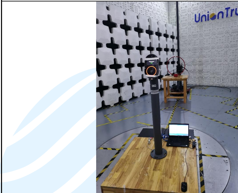
Radiated emission Test Setup (Below 30 MHz)
