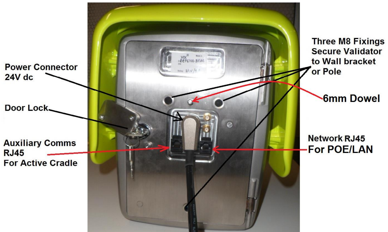
Figure 10: PCP6100 Power and Network connections
