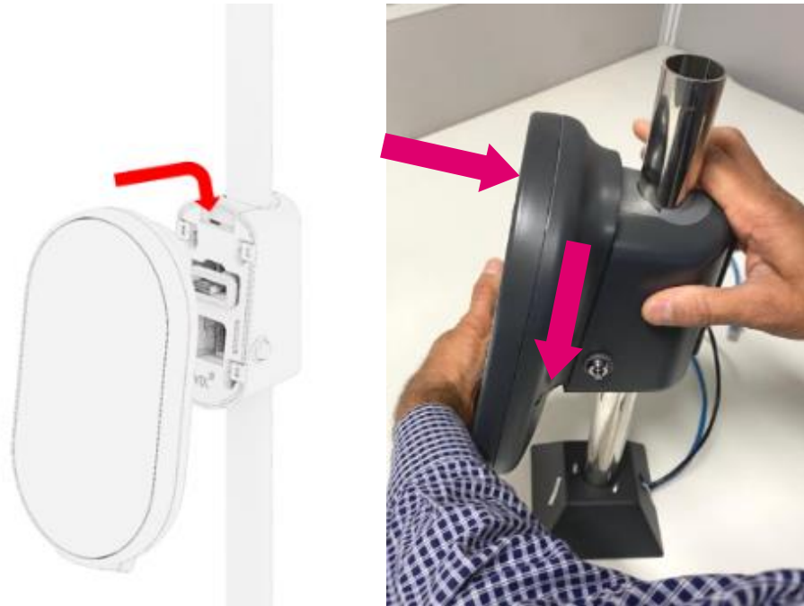
Figure 25: Adept Validator Mounting on Cradle
