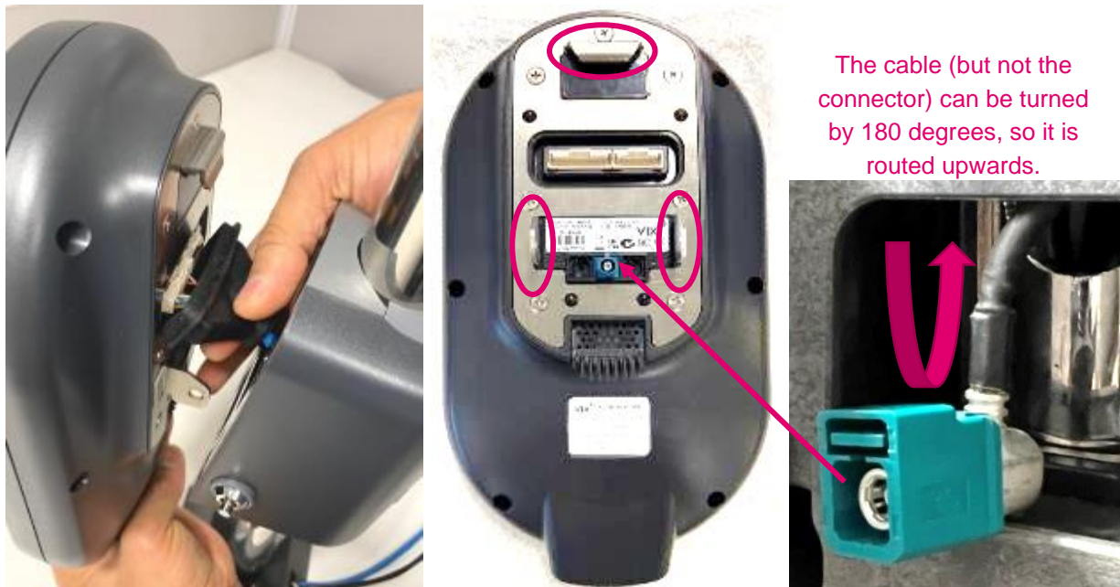
Figure 24: Adept Validator Cable Connections
