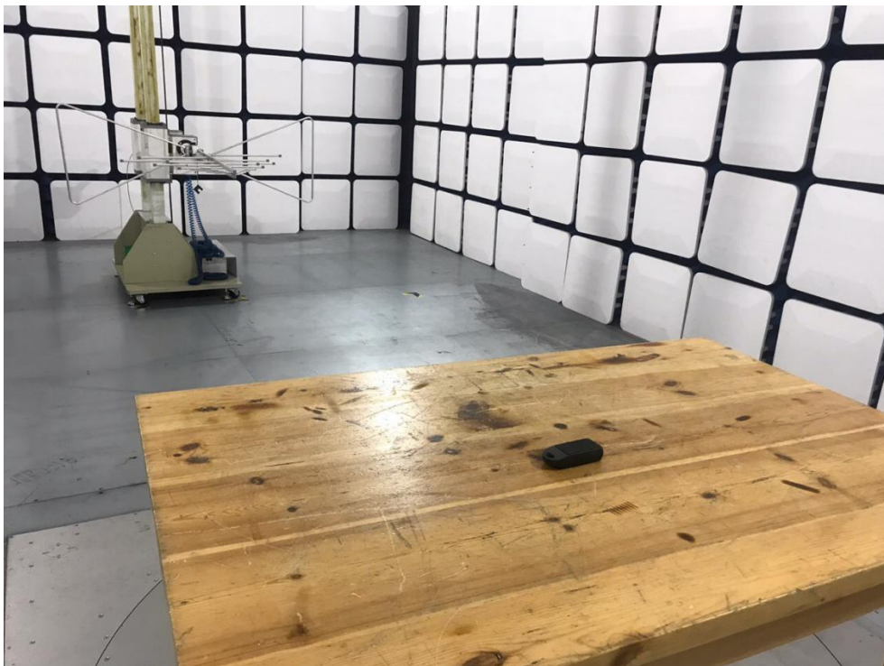
Photo of Radiation Emission Test
