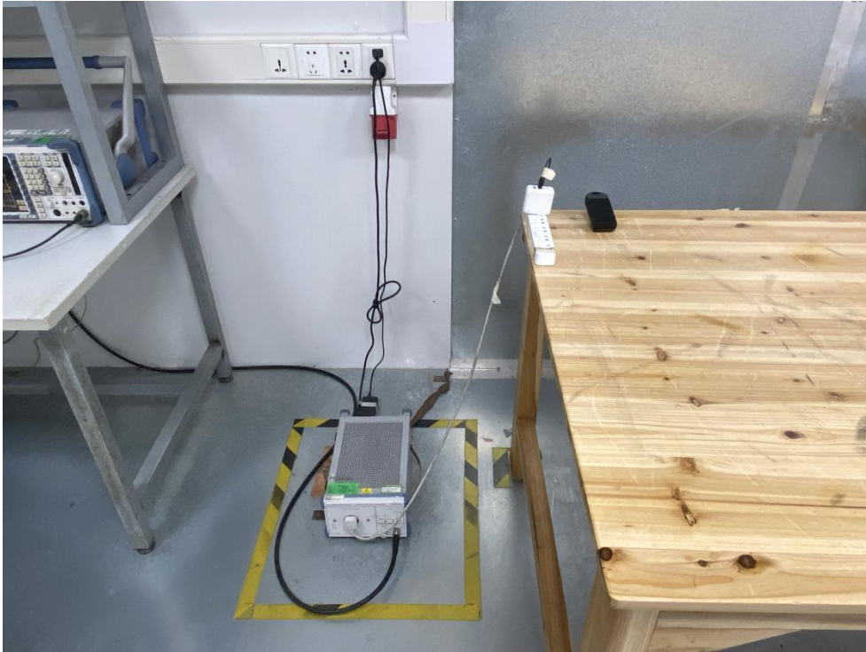
Photo of Conducted Emission Measurement
