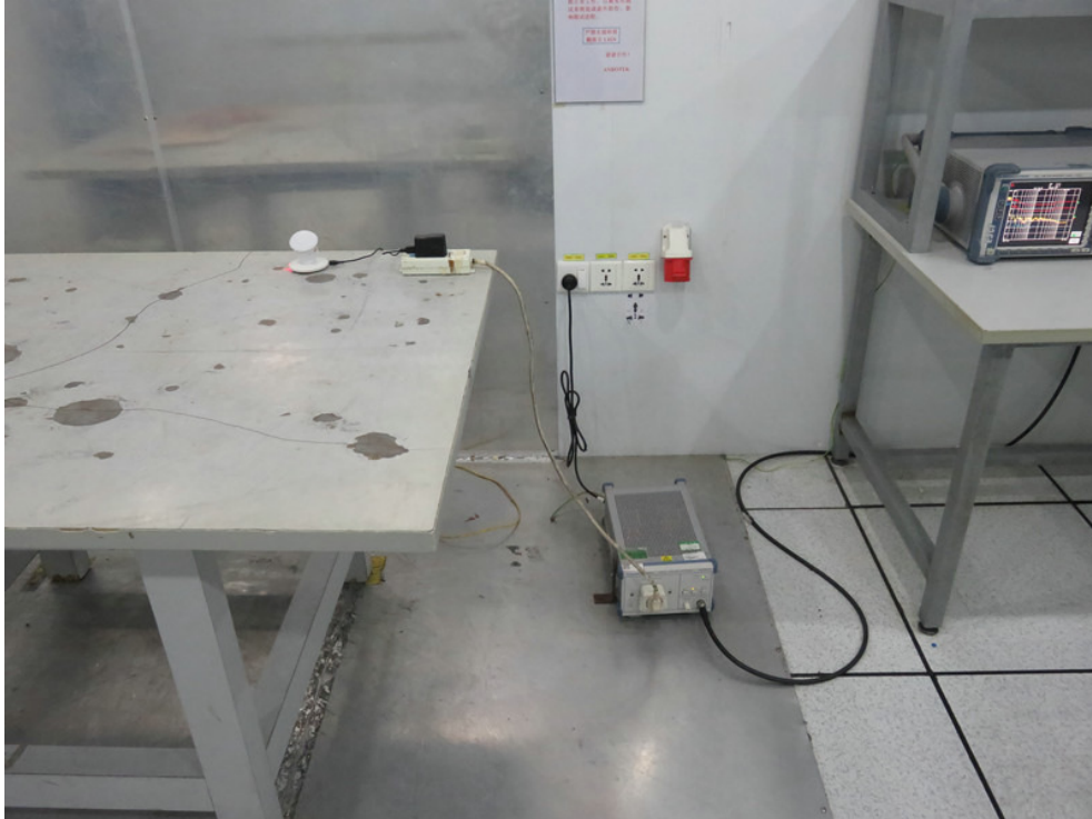
Photo of Conducted Emission Measurement
