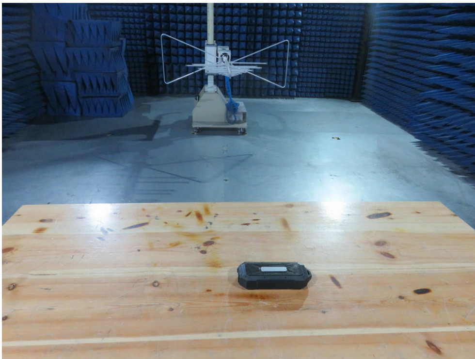
Photo of Radiation Emission Test
