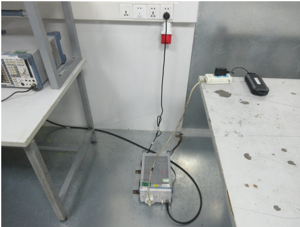
Photo of Conducted Emission Measurement
