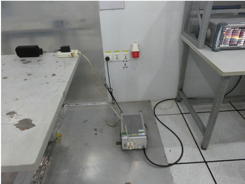
Photo of Conducted Emission Measurement
