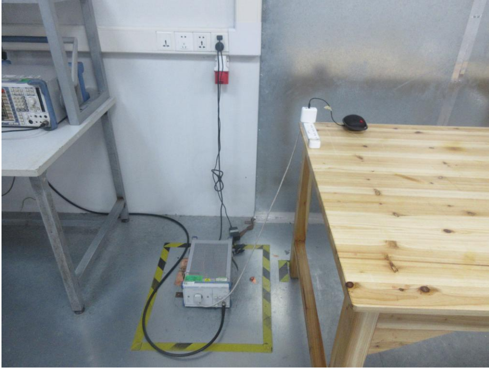
Photo of Conducted Emission Measurement
