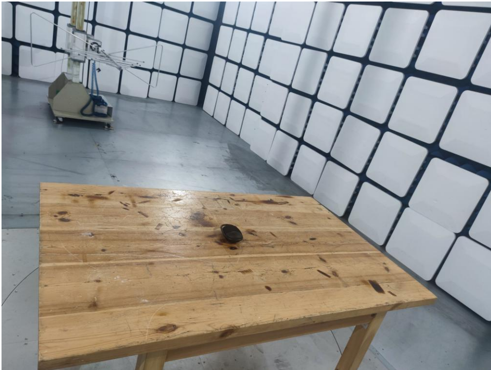
Photo of Radiation Emission Test
