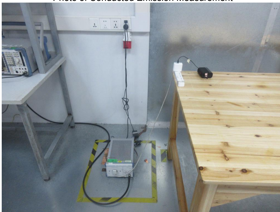
FCC ID: 2AIKE-7197-52 Photo of Conducted Emission Measurement
