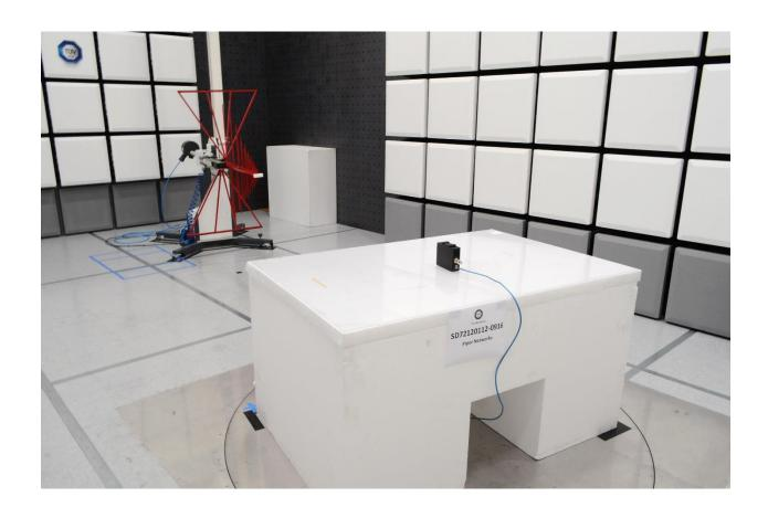
Radiated Emissions Test Setup (below 1 GHz Back)
