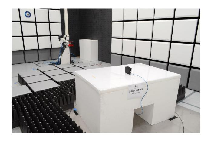
Radiated Emissions Test Setup (above 1GHz Back)
