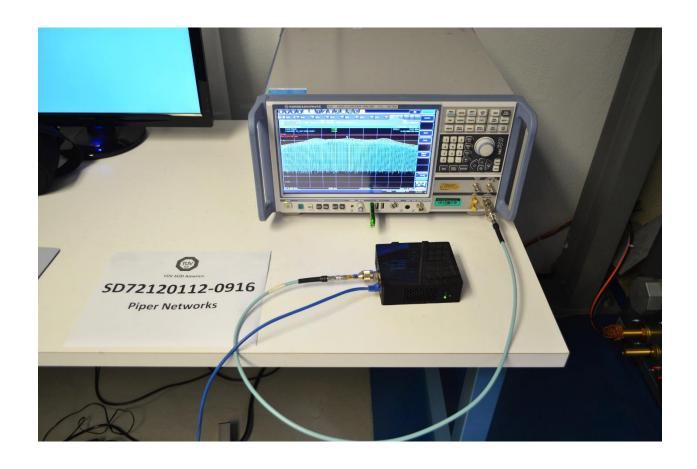
**Conducted Antenna Port Test Setup**
