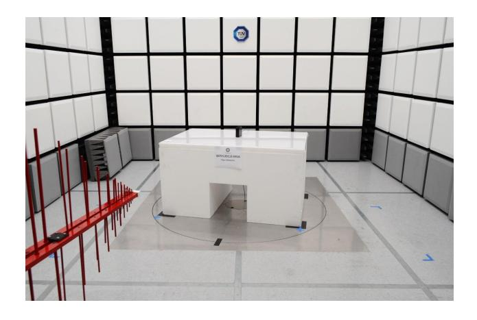
Radiated Emissions Test Setup (below 1 GHz Front)
