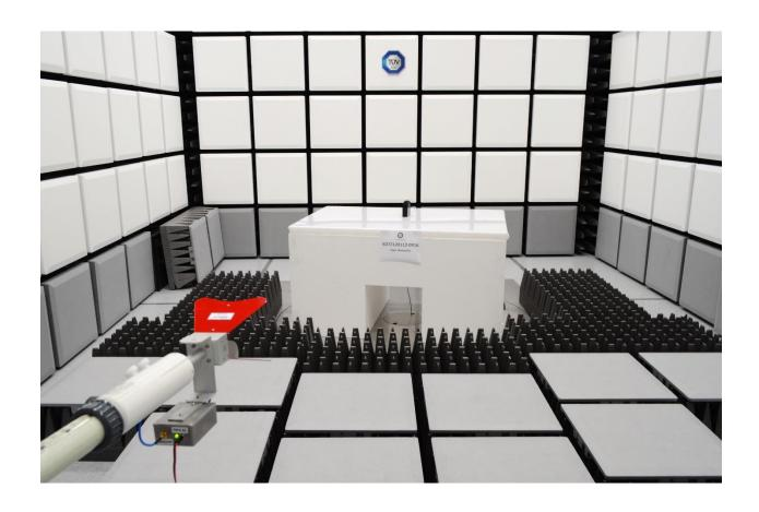
Radiated Emissions Test Setup (above 1GHz Front)
