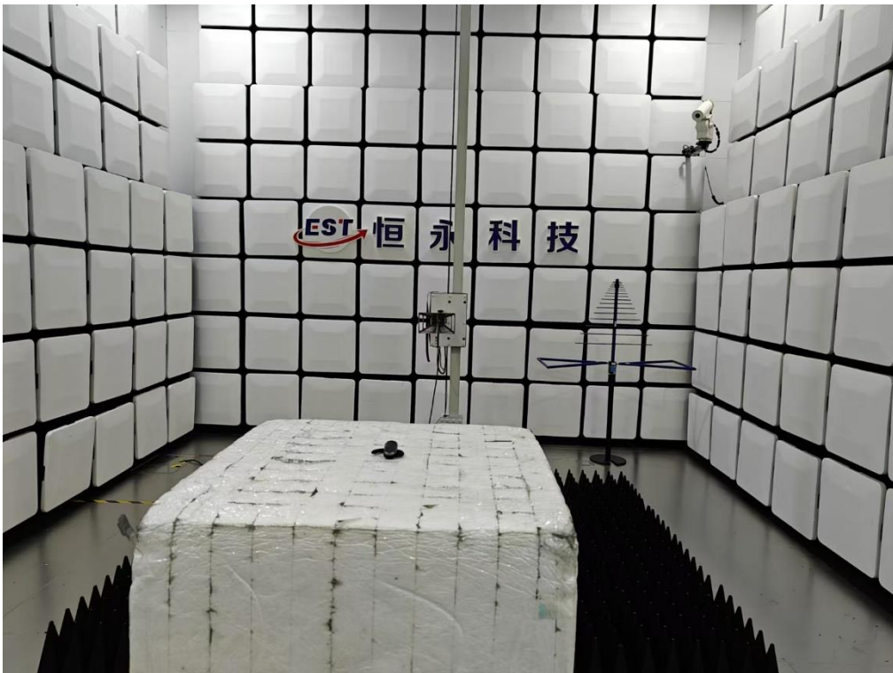
Radiated emission test: Above 1GHz
