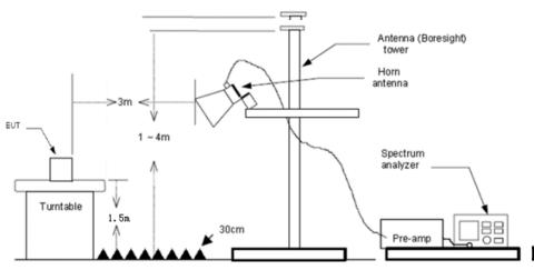
Above 10 GHz shall be extrapolated to the specified distance using an extrapolation factor of 20 dB/decade form 3m to 1.5m.
