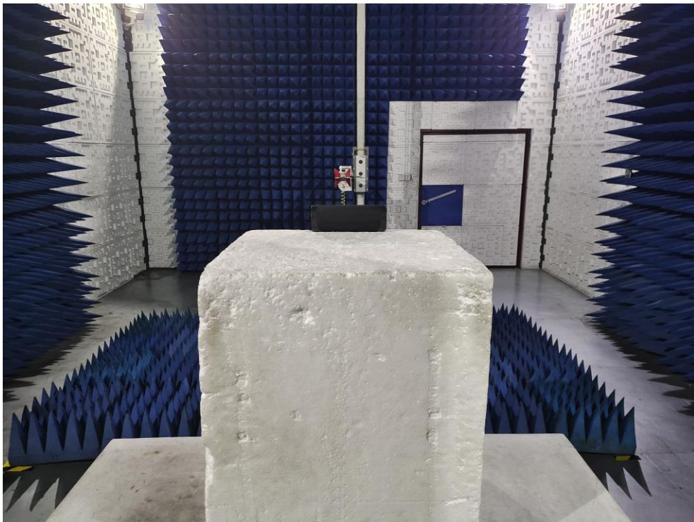
RADIATED EMISSION TEST SETUP ABOVE 1GHz
