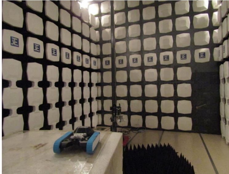
Measurement of Radiated Emission Test Set Up
