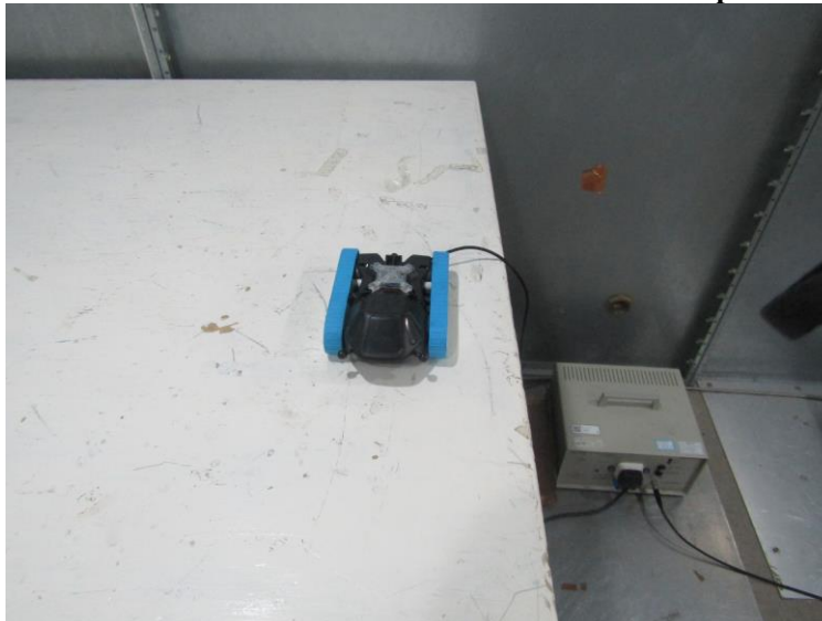
Measurement of Conducted Emission Test Set Up
