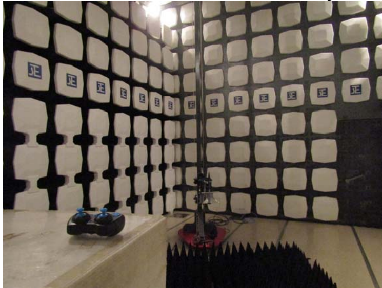
Measurement of Radiated Emission Test Set Up
