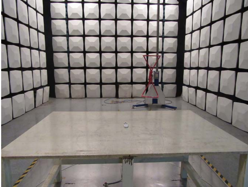
Radiated Disturbance Test Setup View (Below 1GHz)
