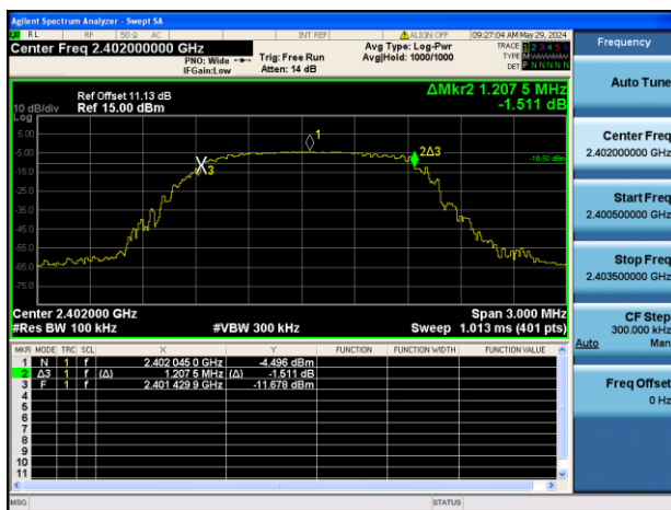
GFSK (BLE 1Mbps) LOW CHANNEL
