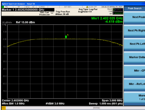
GFSK (BLE 1Mbps) LOW CHANNEL
