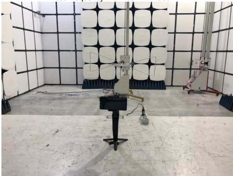
Radiated Spurious Emissions Test Frequency From 30MHz-1000MHz
