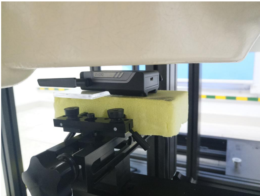
Front face of EUT with ANT B in close at 5mm (180 degrees)
