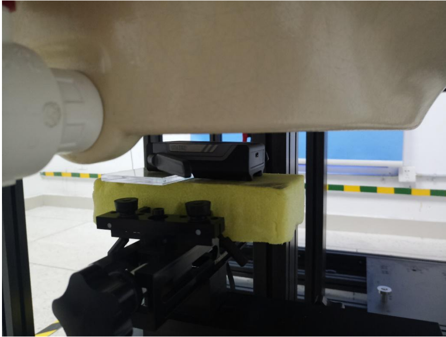
Front face of EUT with ANT B in open at 5mm (45 degrees)
