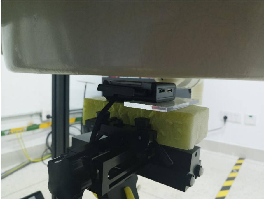
Front face of EUT with ANT A in close at 5mm (0 degrees)
