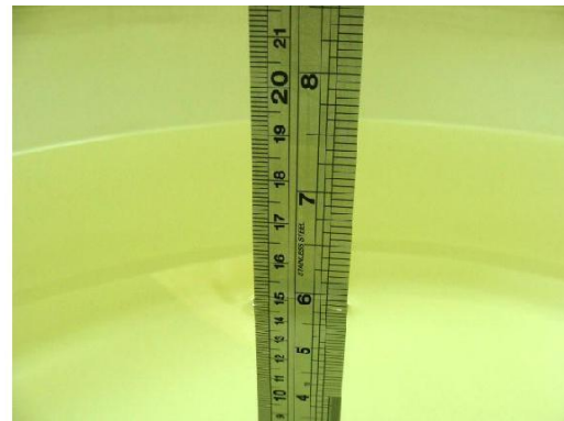
Fig 7.2 Photo of Liquid Height for Body SAR
