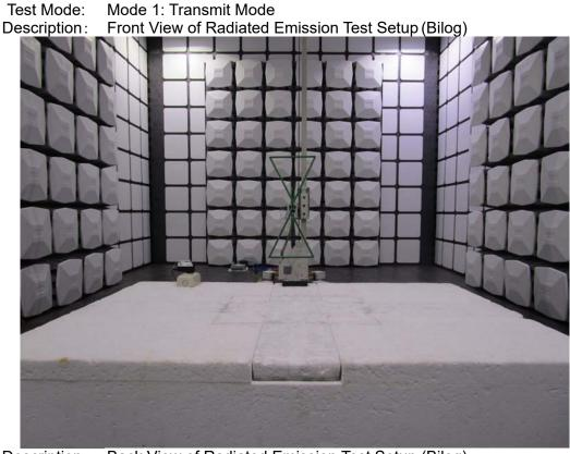
Description: Back View of Radiated Emission Test Setup (Bilog)
