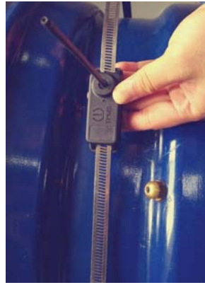
1、 The steel tie around the hub. 2、 Put the sensor on the steel tie 3、 Pre tighten steel tie screw
