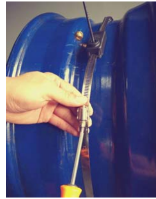
1、 The steel tie around the hub. 2、 Put the sensor on the steel tie 3、 Pre tighten steel tie screw
