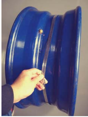
1、 The steel tie around the hub. 2、 Put the sensor on the steel tie 3、 Pre tighten steel tie screw
