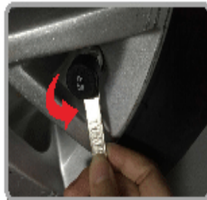
With the tools of lock nut, and ensure close to the sensor
