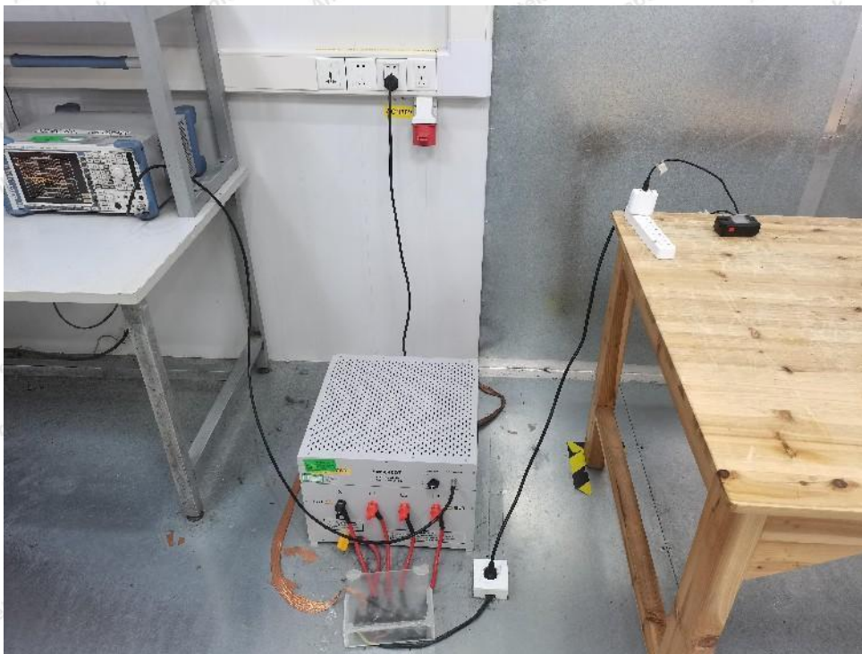
Photo of Power Line Conducted Emission Test
