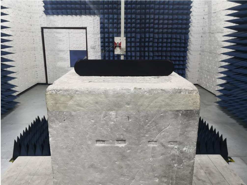
RADIATED EMISSION TEST SETUP ABOVE 1GHZ
