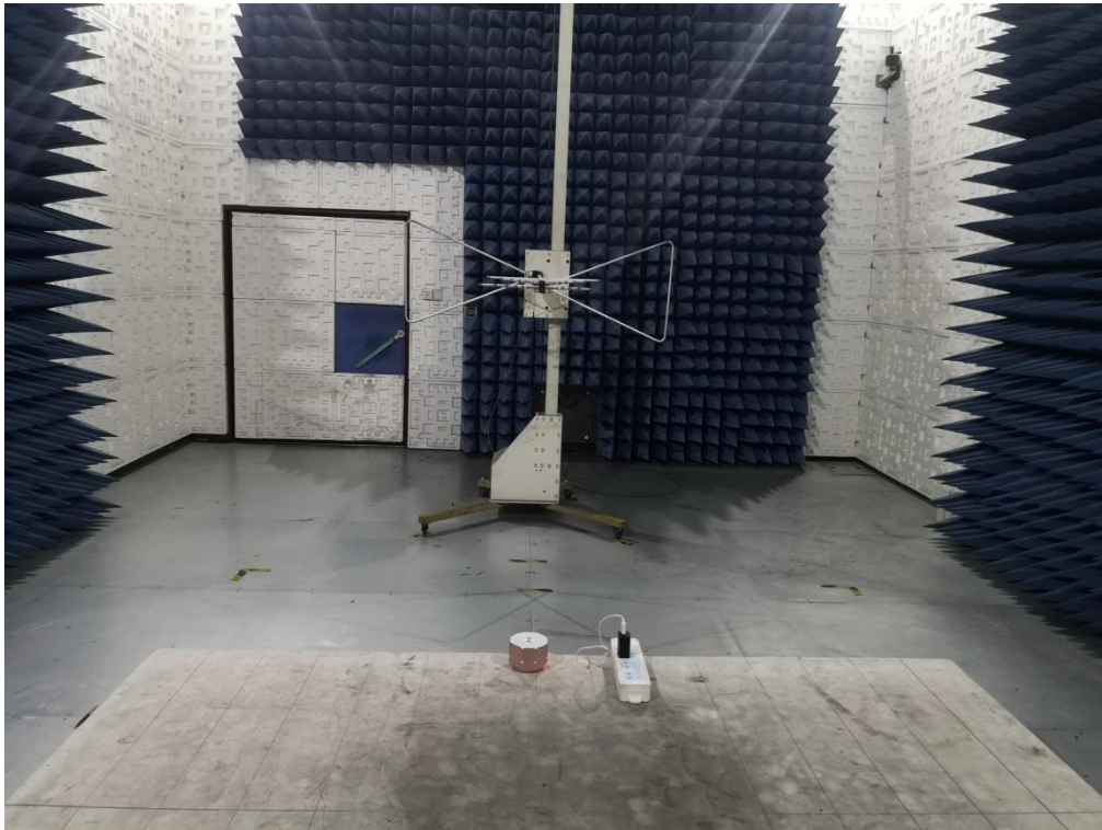
RADIATED EMISSION TEST SETUP ABOVE 1GHz
