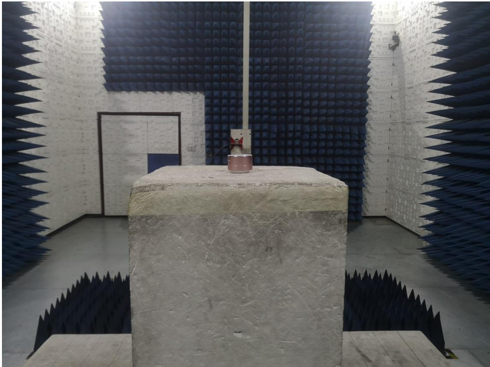
RADIATED EMISSION TEST SETUP ABOVE 1GHz
