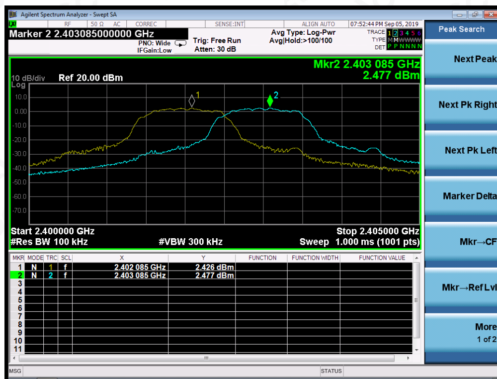
TEST PLOT FOR FREQUENCY SEPARATION
