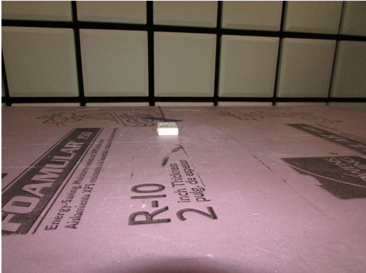
Figure 5: Radiated Emissions – Front – Above 1GHz - XPOS
