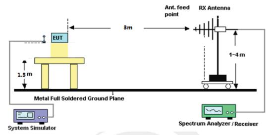
For radiated test from above 1GHz
