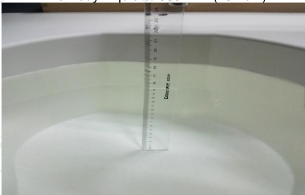
The Body Liquid of 2450MHz (15.3cm)
