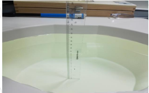
The Body Liquid of 1900MHz (16.4 cm)
