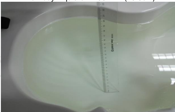
The Head Liquid of 1900MHz (15.5cm)
