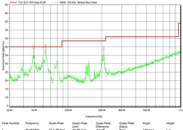
$40 \; dB\mu V/m$ 49.08 MHz  $33.7\;dB\mu V/m$ -6.3 dB Pass 0 Degree 1 m  $37.1 \ dB\mu V/m \ 32.7 \ dB\mu V/m$ 0 Degree 0 Degree 62.916 MHz 40 dBuV/m -2.9 dB Pass 1 m 206.94 MHz 43.5 dBμV/m -10.8 dB Pass 1 m
