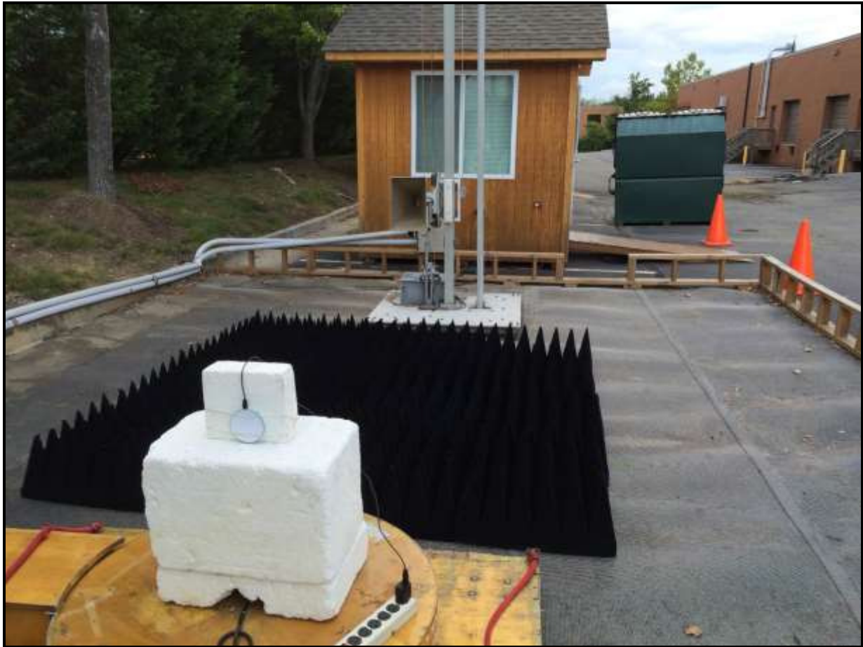
Photograph 2: Radiated Emissions Testing – Front View (above 1 GHz)
