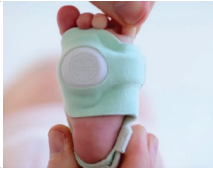
Size 1 newborn sock is always placed with the Sock Electronics on the bottom flat part of the foot .
