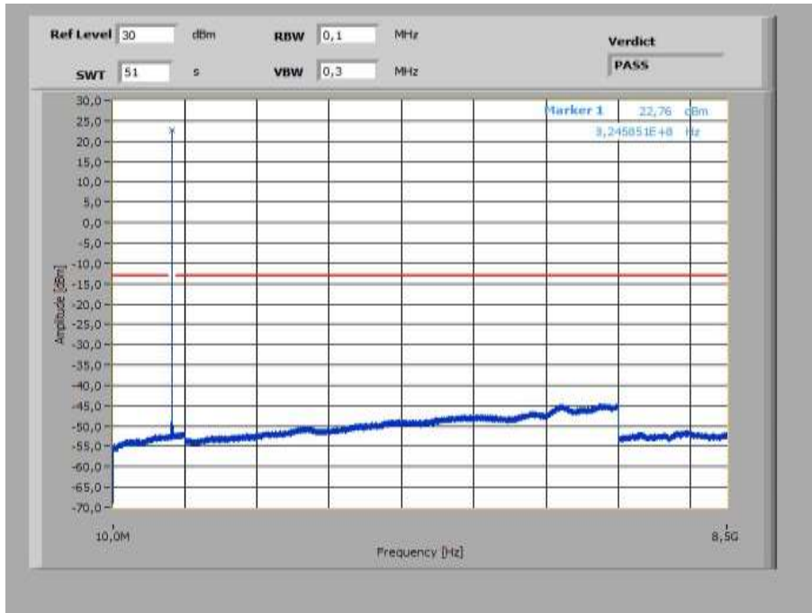
Plot 1: Lowest Channel (10 MHz – 8.5 GHz), spacing 3.75 kHz, 1@0 tones
