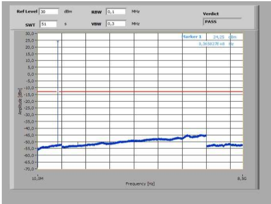
Plot 11: Middle Channel (10 MHz – 8.5 GHz), spacing 15 kHz, 1@11 tones
