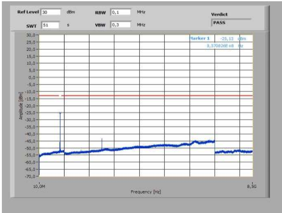
Plot 5: Middle Channel (10 MHz – 8.5 GHz), spacing 3.75 kHz, 1@47 tones
