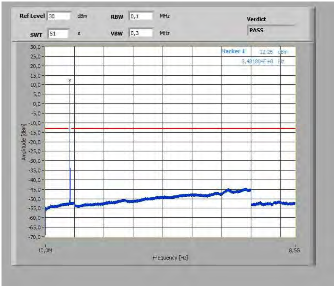
Plot 3: Highest Channel (10 MHz – 8.5 GHz)
