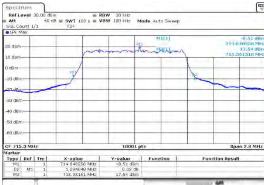
Plot 6: high channel, -26 dBc OBW
