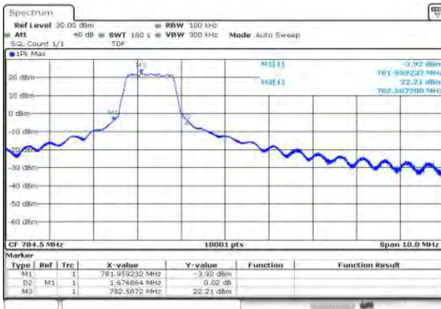
Plot 6: high channel, -26 dBc OBW
