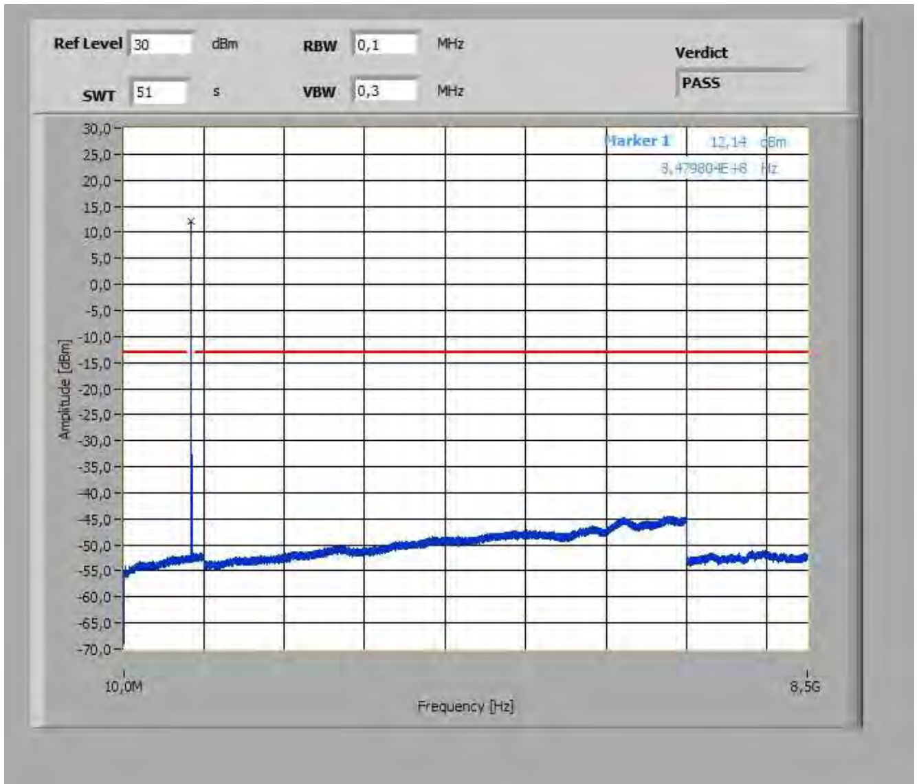
Plot 3: Highest Channel (10 MHz – 8.5 GHz)
