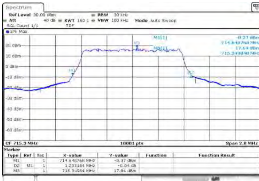
Plot 6: high channel, -26 dBc OBW
