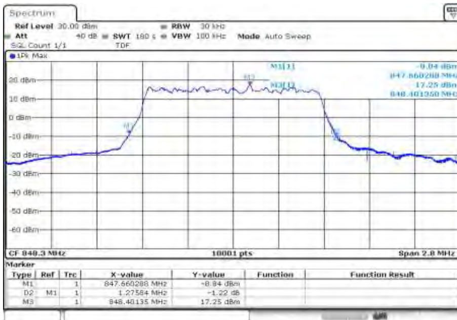
Plot 6: high channel (-26 dBc BW)
