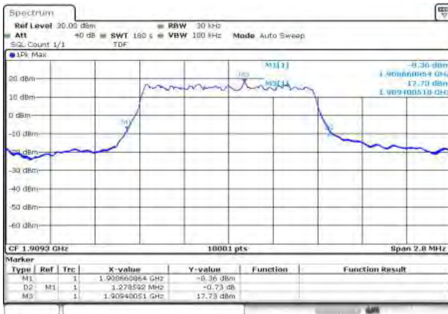
Plot 6: high channel (-26 dBc BW)
