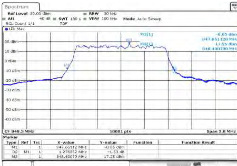
Plot 6: high channel (-26 dBc BW)
