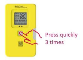
The display starts showing after press quickly 3 times following screen:
