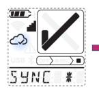
Synchronisation in progress "SYNC" ← Cloud Symbol is blinking
