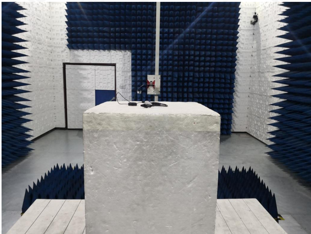
RADIATED EMISSION TEST SETUP ABOVE 1GHZ
