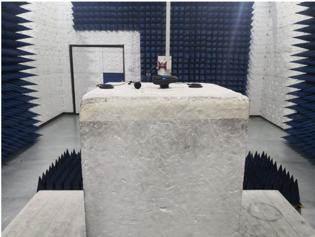
RADIATED EMISSION TEST SETUP ABOVE 1GHz
