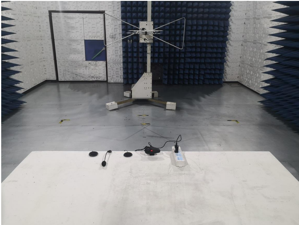
RADIATED EMISSION TEST SETUP ABOVE 1GHz
