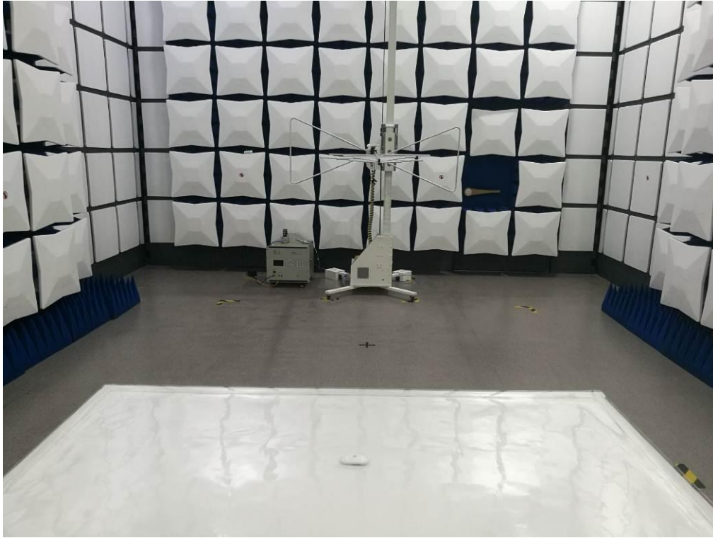
FCC RADIATED EMISSION TEST SETUP
