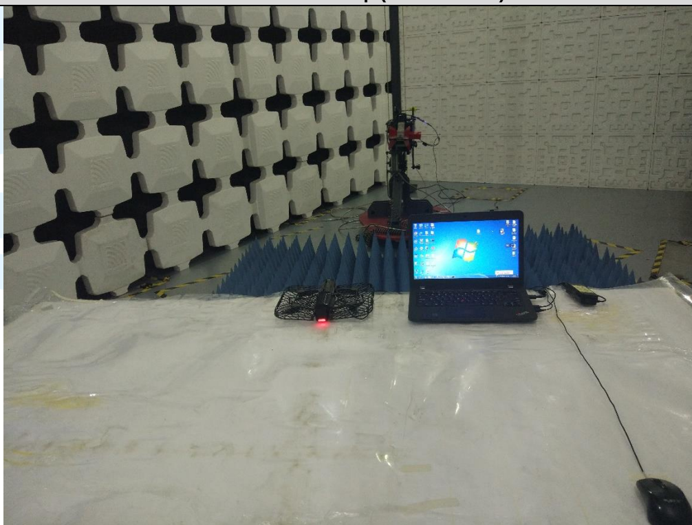
Radiated emission Test Setup (Above 1 GHz) - Mode 4
